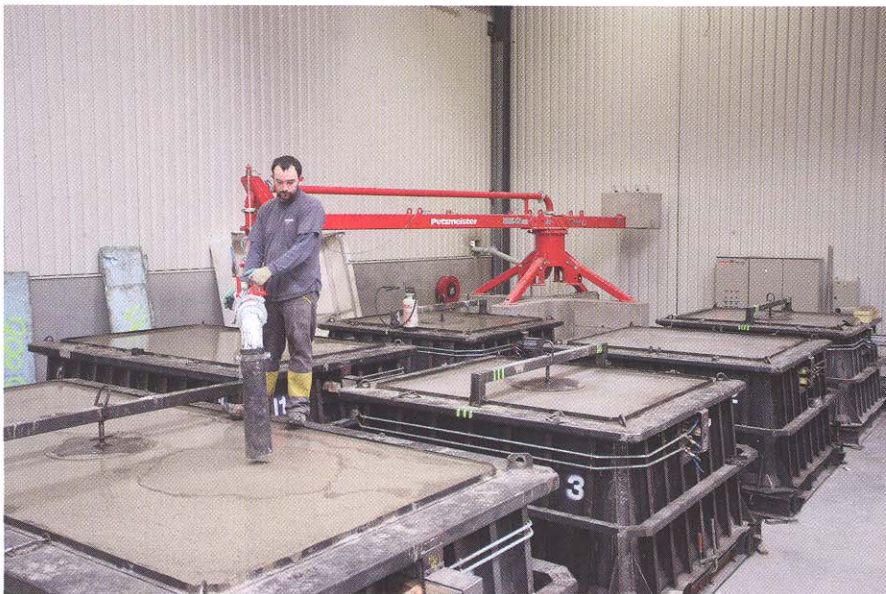
A Putzmeister type RV 13 mechanical spreader was installed for the largest receptacles (10,000 up to 20,000 litres)
