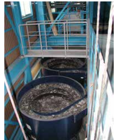
Installation example of 2 pcs MD500 in Japan. Dual dosing equipment for optimisation of steel fibre concrete production for flooring and shotcrete.
