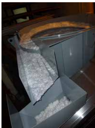
Dosing system MD400 with weigh-belt High precision dosing of micro synthetic fibres. Dosing accuracy: \pm 10 g
