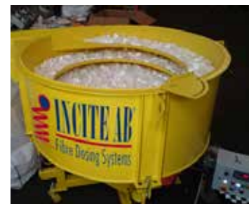
Dosing unit type MD75 Installed in CERIB - central concrete institute, France.
