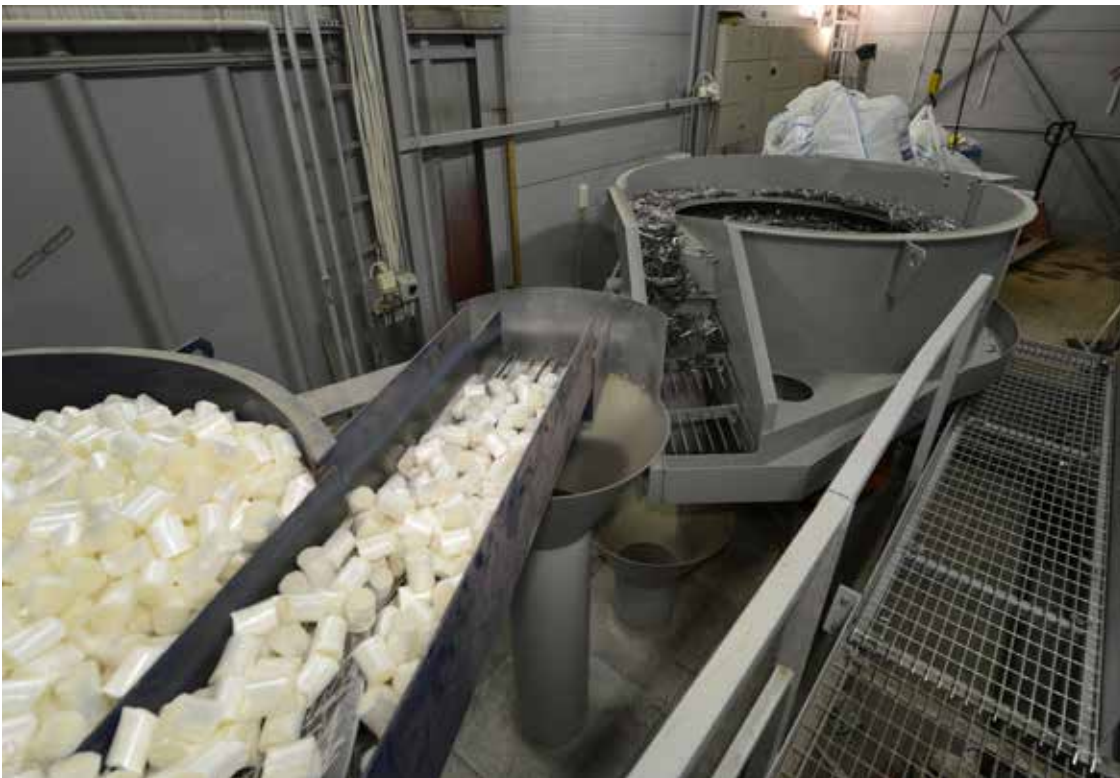
Dosing unit type MD500 + MD1200SR in Finland Dual dosing equipments for dosing of macro synthetic fibres in pucks and steel fibres.
