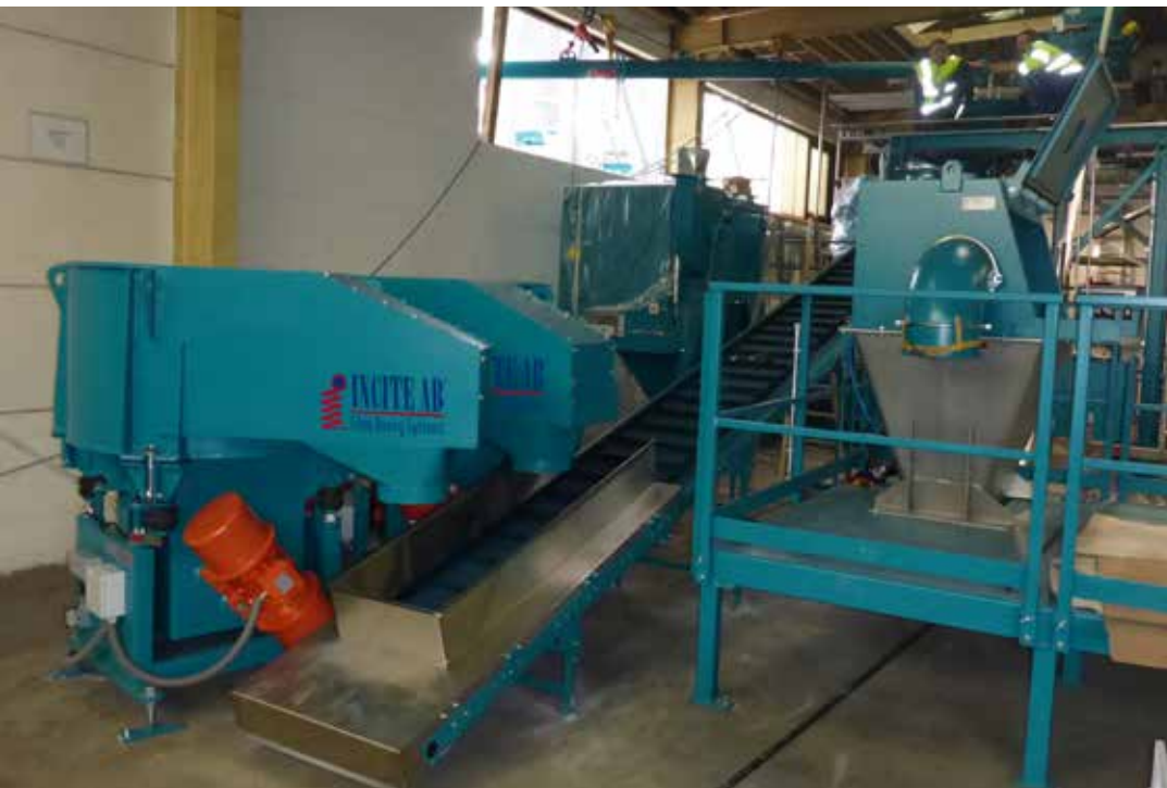
Installation example of 2 pcs of model MD250SR in Germany. Dosing two different types of micro steel fibre with dosing speed at 25 kg/min.
