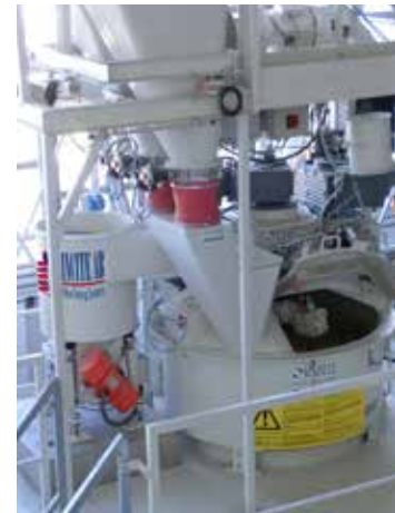
Dosing unit type MD75 Installed in CERIB - central concrete institute, France.
